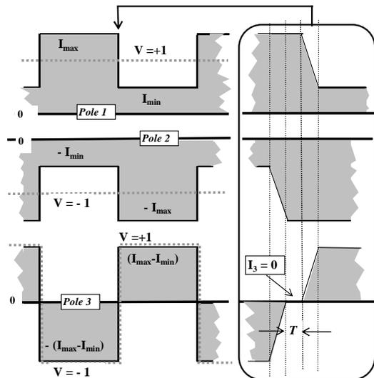
Figure 2 Current-time diagram of current in Poles 1, 2 and 3.
