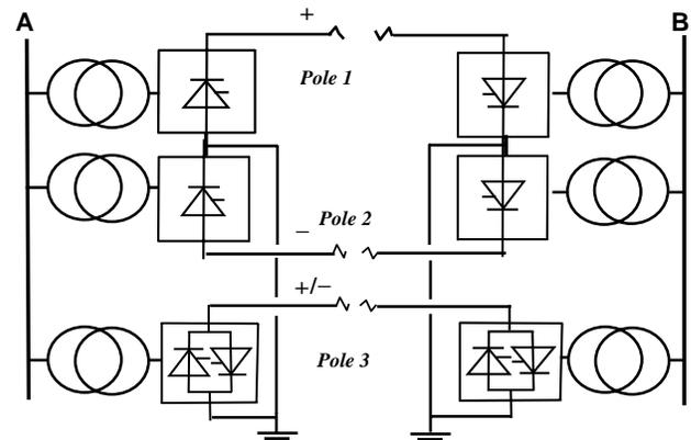
Figure 1 Parallel bipole and monopole HVDC systems.
