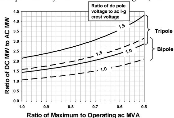
Figure 3 Example range of expectations in AC to DC transmission line conversion.
