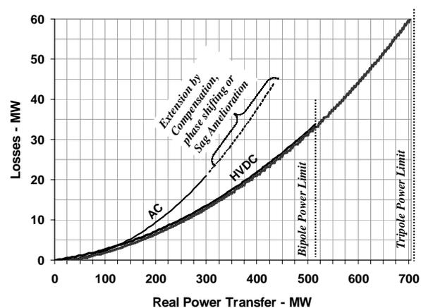
Figure 4 Comparison of ac and dc losses for equal power levels.
